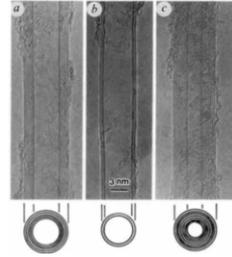
Fig. 1 Electron micrographs of microtubules of graphitic carbon, parallel with the c-axis, showing the (100) lattice images of graphite. A gross effect on the wall thickness is illustrated. a, The cross-section of the graphitic sheet, diameter 0.7 nm. b, The sheet tube, diameter 5.5 nm. c, Seven-sheet tube, diameter 0.5 nm, which has the smallest hollow diameter (2.2 nm).
